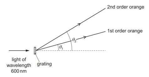
What is the angular separation  $(\theta_2 - \theta_1)$  between the first and second order maxima of the orange light?
