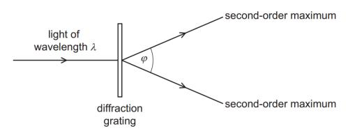
The angle between the two second-order maxima is  $\varphi$ .
