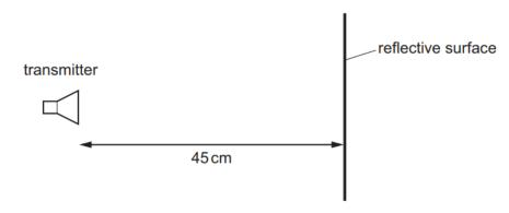
The emitted waves have a frequency of 1.00 GHz. A stationary wave is produced with a node at the transmitter and a node at the surface.
