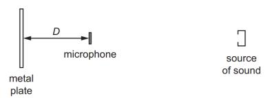
Sound of the unknown frequency is reflected back from a metal plate. A microphone placed at a distance D from the metal plate detects the sound intensity. A minimum intensity is detected with  $D = 12.0 \,\mathrm{cm}$ . The plate is moved further away from the microphone until the next minimum is detected with  $D = 15.0 \,\mathrm{cm}$ .
