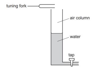
The tube is filled and then water is allowed to run out of it. The first two stationary waves occur when the air column lengths are 0.14 m and 0.42 m.
