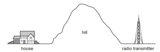
The radio transmitter cannot be seen from the house, but radio waves from the transmitter are received at the house.
