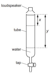
A tap at the bottom of the tube is opened so that water slowly leaves the tube. For some lengths of the air column in the tube, the sound heard is much louder.
