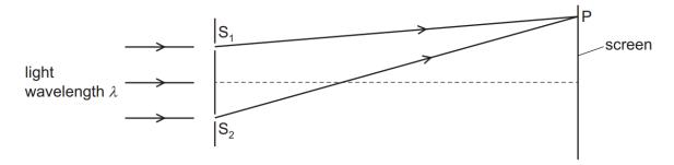
The *n*th **dark** fringe from the central bright fringe is observed at point P on the screen.
