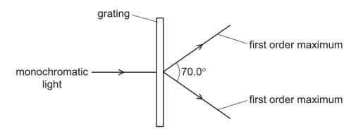
The spacing of the slits in the grating is  $1.00\times10^{-6}\,\text{m}$ . The angle between the first order diffraction maxima is  $70.0^{\circ}$ .
