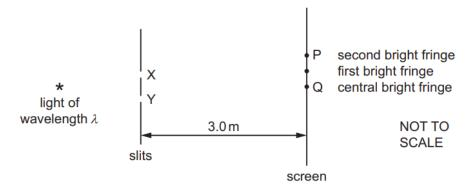
An interference pattern is observed on a screen 3.0 m away from the slits X and Y, which have a separation of 1.0 mm.
