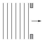
Some diffraction of the water waves is observed.
