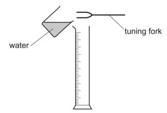
Water is then gradually poured into the measuring cylinder. A much louder sound is first heard when the water level is 2.9 cm above the base of the measuring cylinder. A second much louder sound is heard when the water level reaches a height of 67.3 cm above the base.
