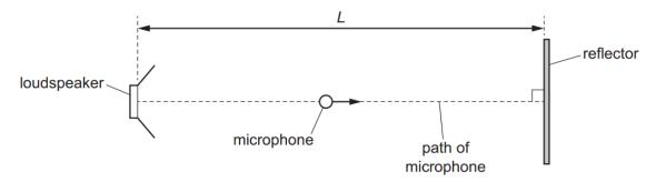
A stationary wave is formed with an antinode at the loudspeaker. A microphone is moved from the loudspeaker to the reflector.
